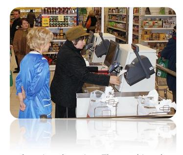
and paying the price. The machine does the rest. It controls weight of products in order to identify the product, which has not been scanned. It is also responsible for credit card or cash payment.
